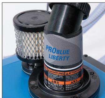
*Adhesive inlet tube and air filter*
